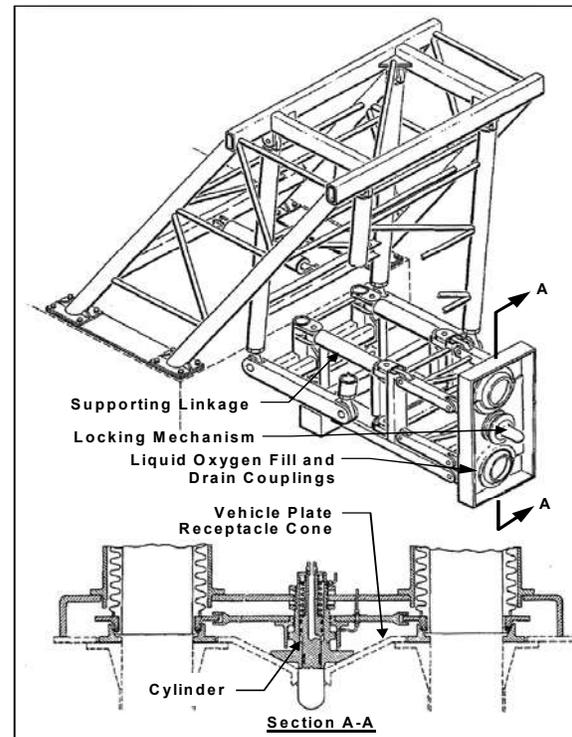
Figure 15. Self-aligning Umbilical (Saturn V – SIC Intertank)
