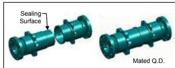
**Figure 19. Slip on Type Quick Disconnect**
