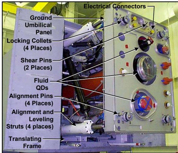
**Figure 2. Subassembly / Component Overview**
