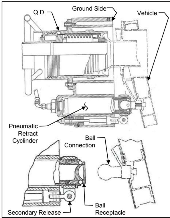
**Figure 16. Ball-Locking Type Mechanism**
