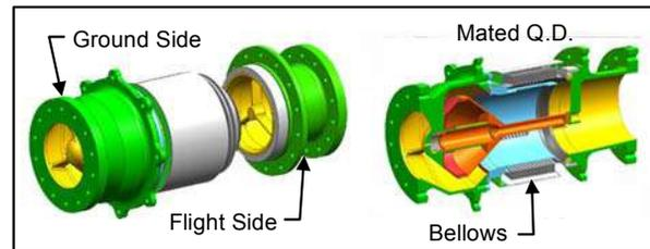
**Figure 18. Bellows Type Quick Disconnect**
