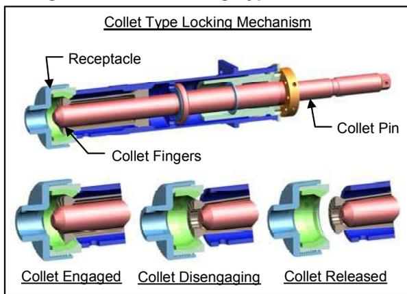
**Figure 17. Collet Type Locking Mechanism**
